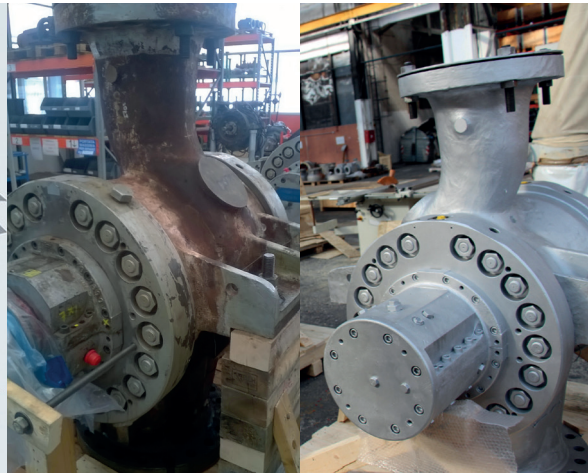
Embalse project - Argentina - main feed water pump before (left) and after (right) refurbishment at Termomeccanica Pompe's Italian facilities
