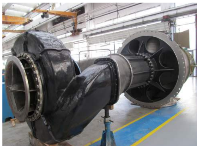
Assembly of Termomeccanica condensate extraction pump to be installed in the Enel Green Power Larderello power plant
