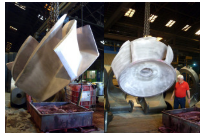
Impeller during non destructive testing phase.
