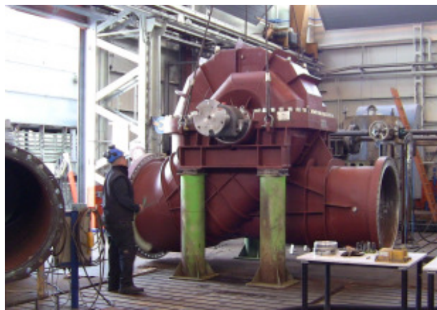
fig.1 - DD pump test preparation in Termomeccanica's in-house test center
