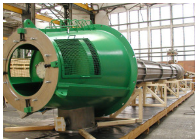
SWP per Zhuhai LNG Receiving Terminal before delivery
