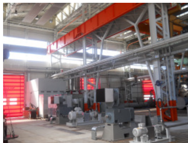
New Test Rig for API 610 Pumps Type OH2, BB2, BB5, VS1, VS4 and VS6.
