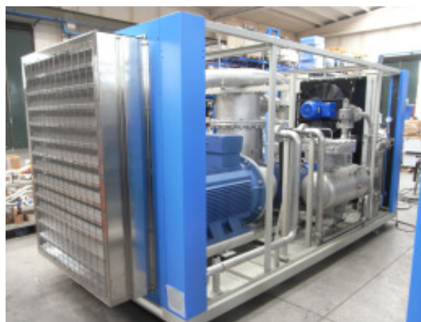
Biogas compression skid
