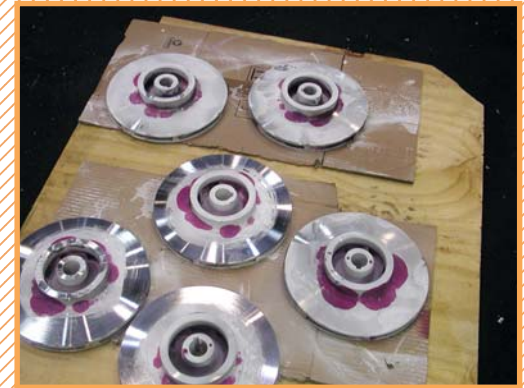
Non Destructive Tests on Impellers
