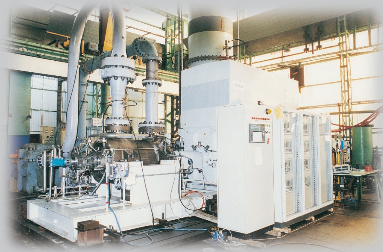
Test loop in hot condition of barrel feed water pump
